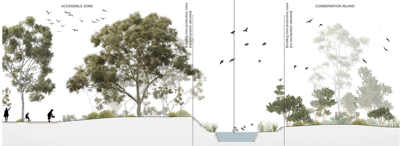
Conservation Island - cross-section showing narrow water barrier with Ha-Ha walls.
